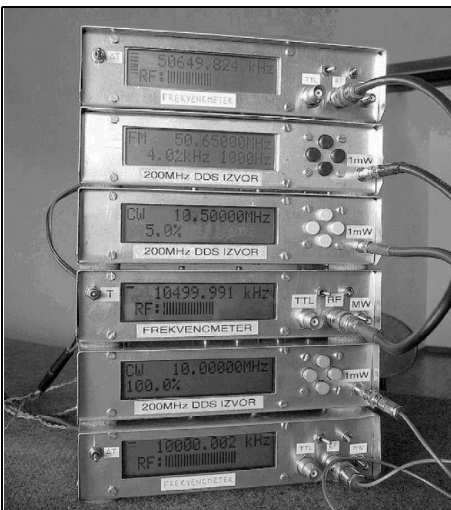
Fig 5: Three signal generator prototypes under test.
